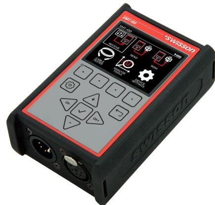
Signal testing helps to check for signal integrity, providing real-time insights into the flow of data packages and monitoring timing aspects of DMX & RDM signals. For physical infrastructure, the cable testing feature automatically scans all pin connections in any 3-pin or 5-pin DMX cable.
