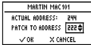
A device which has not been patched yet, is displayed with the DMX address in brackets. As soon as the device is patched the brackets disappear.
