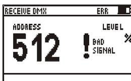
If the DMX can't be decoded by the XMT, BAD SIGNAL will be shown instead of the value.
