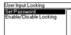
When the device is locked, the user will only be able to see the Home Screen (see page 8) and the Ethernet Port Status Information (see page 24). Since the menu is unavailable while the device is locked, the Ethernet Port Status Information is only accessible via the Ethernet port button [E].
